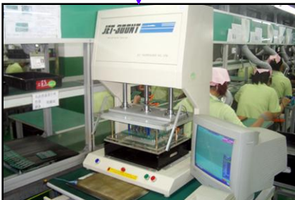
PCB ICT test (In- Circuit-Test)
