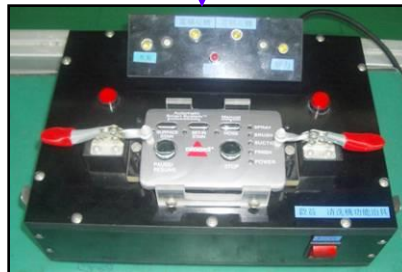
MCU PCB semi-finished goods function test
